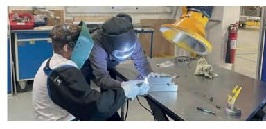
containing all the parts for their own mini conveyor. Under the watchful eye of our expert welders, they were guided and taught to mark, drill holes, and weld the frame together, eventually completing the mini conveyor each of them walked out with at the end of the day. Once the frame was welded, sanded, and polished, the students delved into the assembly manual that guided them through assembling the automation part and finally getting the conveyor belt to run.
